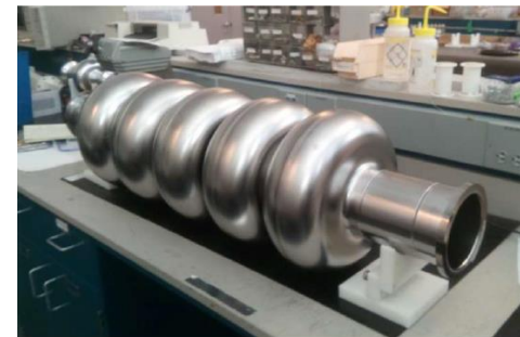
The first fabricated Nb 801.58 MHz 5-cell elliptical cavity at JLab.
