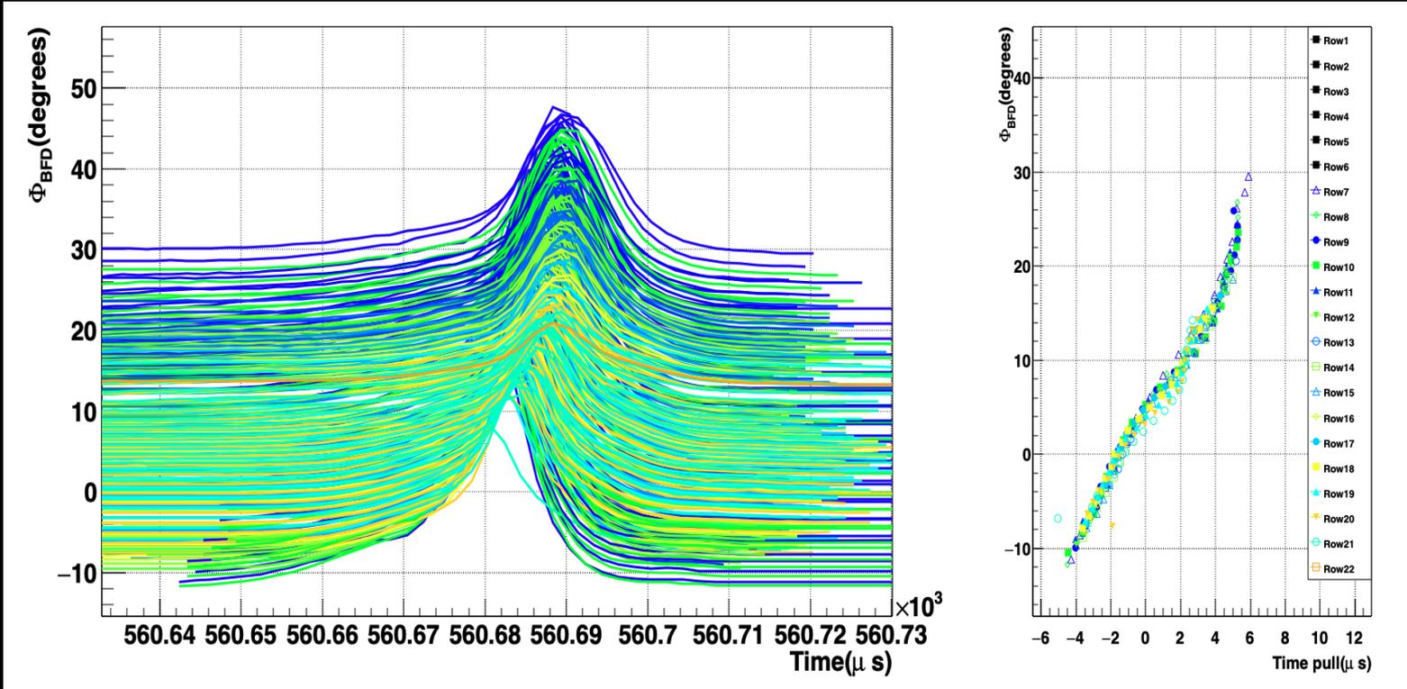
ELVES traces for all pixels realigned at source location, vs azimuth with respect to the vertical plane joining FD and lightning source location from ENTLN reconstruction (5km away)
