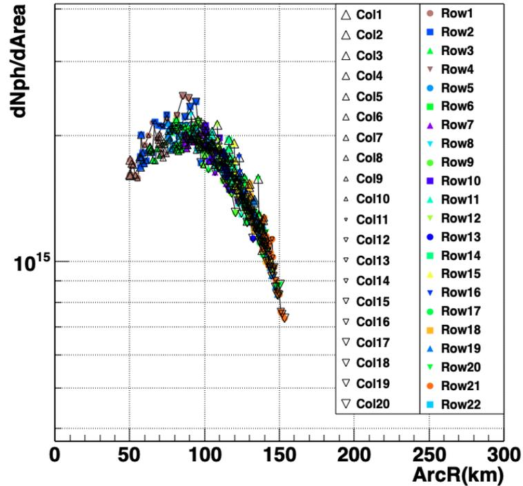
Light intensity distribution vs arc distance from lightning location
