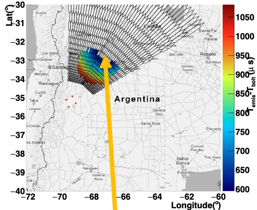
After correcting for time delay, the center is at the lightning source location
