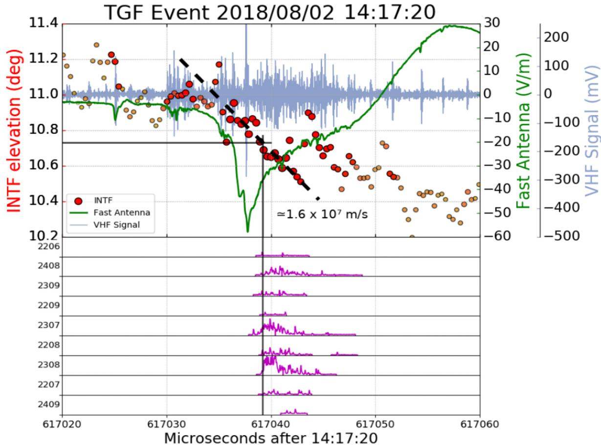
The black vertical line shows the median onset time of the TGF relative to the INTF and fast antenna data. Purple traces in the lower panels are particle detector responses. The detection times are in good agreement with one another as well as the median, indicating the onset time of the TGF during the spheric and the VHF radiation development.
