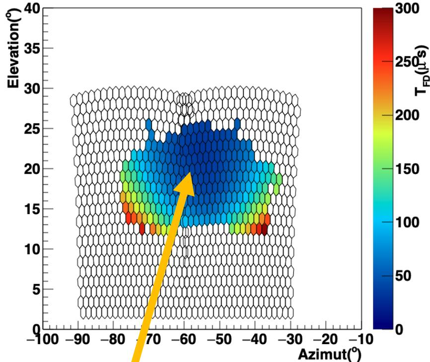
Here the center is in the direction with the shortest path between source and FD
