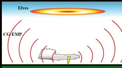
A vertical lightning is like a radiating dipole (Hertz)
