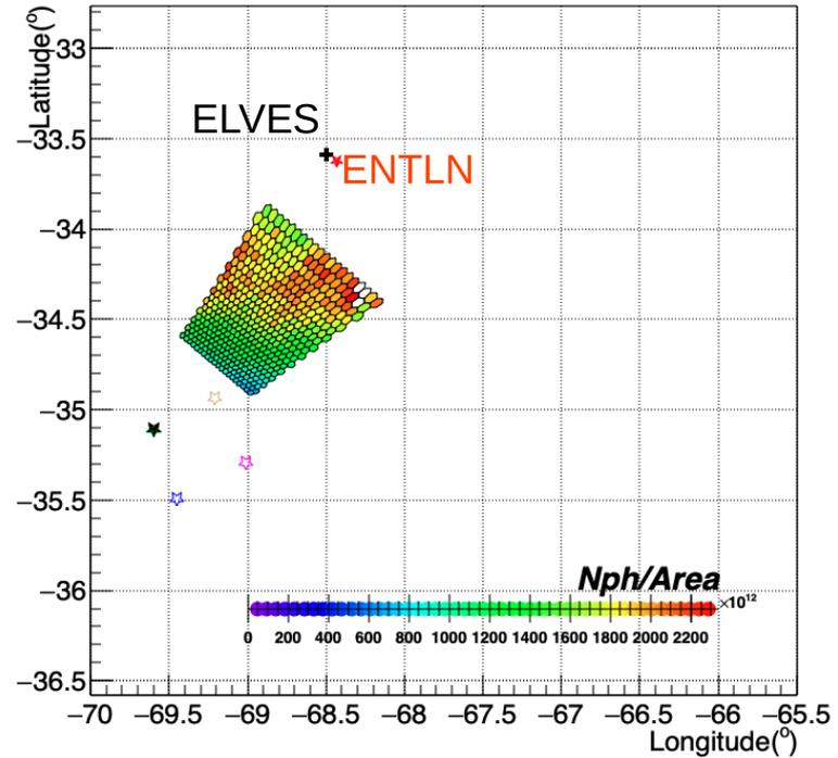
Reconstruction of lightning source location from Auger based on a 3D time fit of ELVES signals
