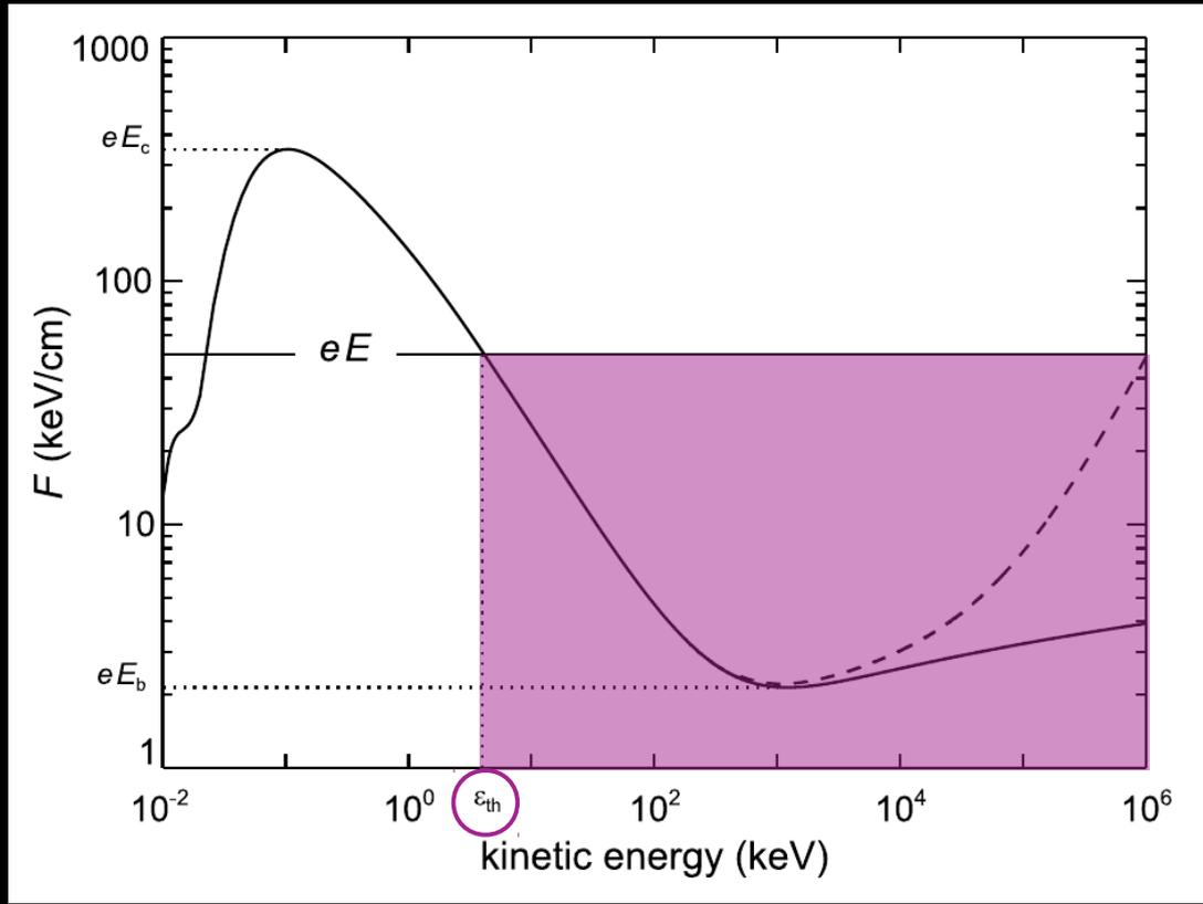
Figure shows the effective frictional force or rate of energy loss of an energetic electron moving in air.
