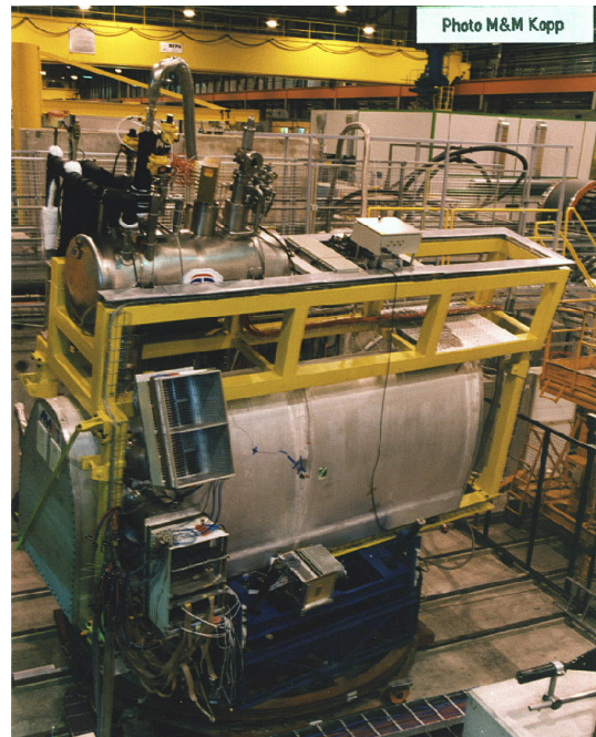
Figure 8 : module 0 in testbeam at CERN in 1999 in its dedicated cryostat.
