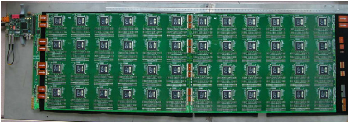
Figure 133 : \mu egas detector of 32 \times 96 \text{ cm}^2 designed by LAPP and readout by 96 HaRDROC2.
