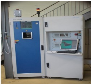
REALIZER SLM300-400W 300x300x300mm
