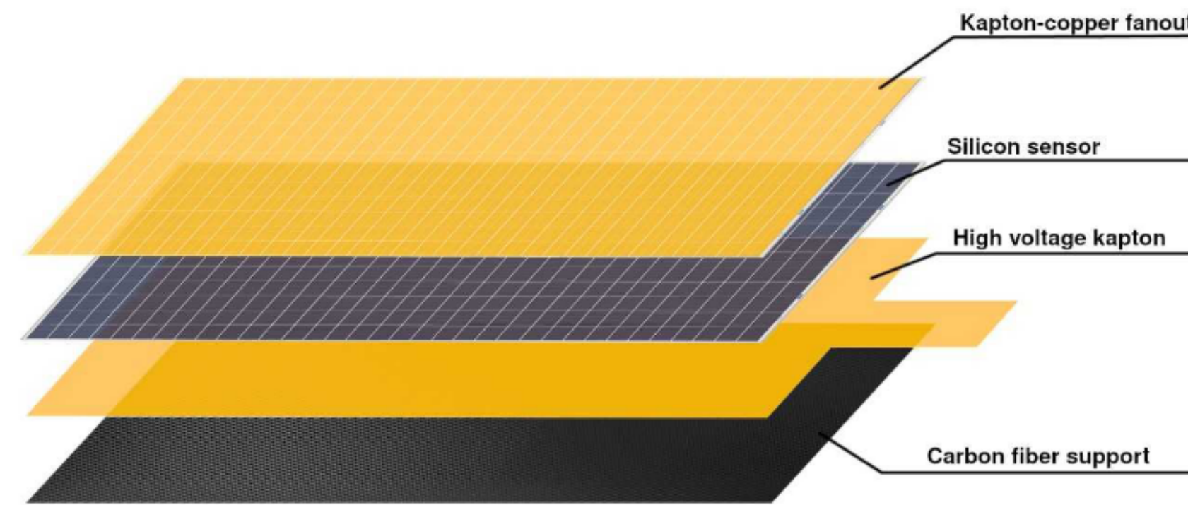
High-granularity ECAL layer
