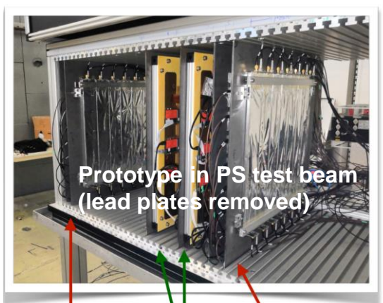
2 scintillator layers (x & y) 2 Micro-Megas 2 scintillator layers (x & y)
