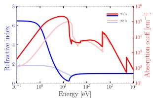
Refractive index and absorption coefficient for Ti illuminated by a XFEL pulse of I= $10^{17}$  W/cm<sup>2</sup>, FWHM=30 fs and h $\nu$ =6 keV.
