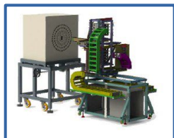
BEta-deLayEd Neutron detector (BELEN) 48 ^3\text{He} cylindrical counters
