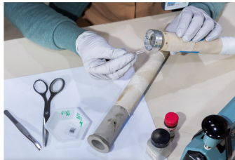
Li-plastic target holder Teflon sample support
