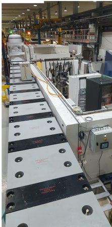
LN2 line, detectors cooling on structure, cabling and electronics connection
