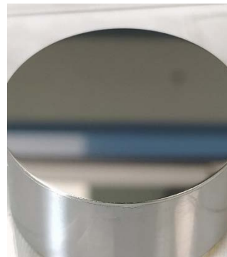
Polished surface (Low waviness, low roughness)
