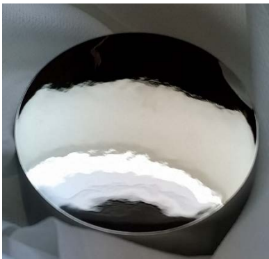
Etched surface (High waviness, low roughness)
