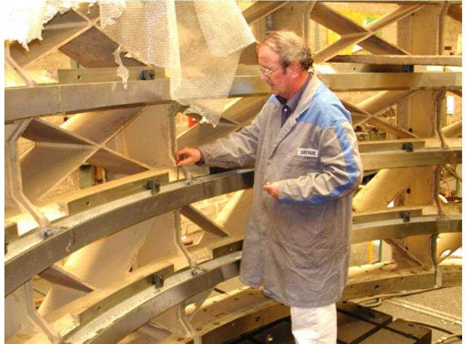
Outer rings machining at the company. large diameter, high accuracy
