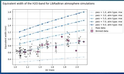
Precipitable water vapor quantity measurement via the equivalent width of the 720nm absorption band
